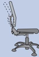
The backrest should be tilted slightly back so the angle of the trunk is five to 15 degrees from vertical. There may also be a lever that allows the backrest and seat to rock back and forth. This “rocking chair” mechanism can be used occasionally to take some of the loading off the low back.
