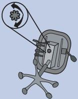
This is usually a round knob on the underside of the seat that will increase the tension in the backrest. If there's a lot of play in the backrest when you lean back, the tension knob should be tightened.
