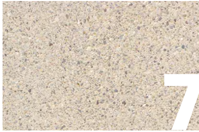
EXPOSED AGGREGATE CONCRETE
