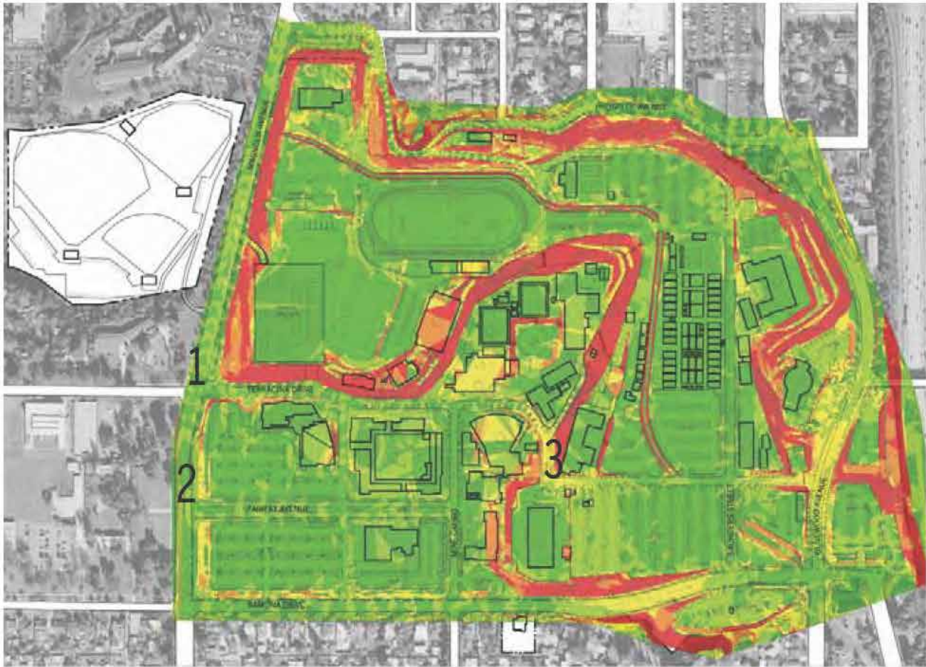
FIGURE 2-21. Slope analysis of existing slope percentages
