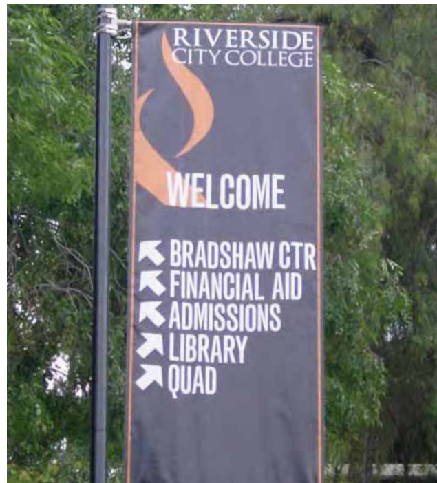
Banner signs are not the proper height for vehicle directionals
