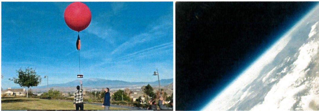
Fig. 2: (i) The launch of the MVC weather balloon with a small payload in 2015. (ii) Earth's curvature is clearly seen in this photo taken by the video camera in the payload. The altitude is just over 100,000 feet. Note the dark sky in absence of atmospheric scatterings.
